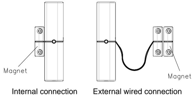
Choose either the internal or external wired connection, both of which types cannot be in existence at the same time.
