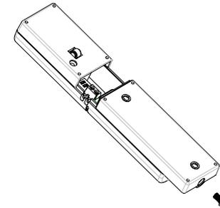
2. Fit 3 1.5V AAA batteries supplied to the battery compartment.
